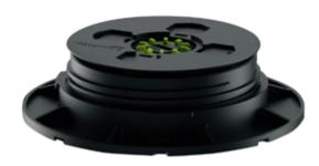
The Uptec SUPAS pedestal is adjustable in height from 43 to 58 mm (1-11/16" - 2-9/32"), with a base diameter of 190 mm (7-31/64") and a head of 130 mm (5-1/8").
